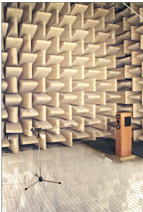
VISATON's anechoic chamber
