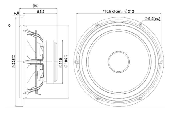
Measuring conditions: Factory new driver, "broken in" 30 min. Half space free-field (2 pi) above 100 Hz. Anechoic room 6x7x8 meters. IEC specs. refer to IEC 60268-5 third edition. All EAD products are RoHS compliant. Sensitivity/2.83V/1m/ 300-1000Hz.
